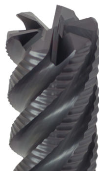
430 SERIES 4 & 6 Flute 40° Helix Negative Rake Angle S Varianta Supral Coating
