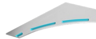
Stitch bead Hybrid joining
