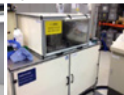
Impulse pressure test stand up to 4000 bar
